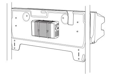
7. Align mounting slots on bottom of cradle with studs on plate.
