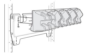
7. Secure cradle to plate using two M5 safety screws (provided with plate).
