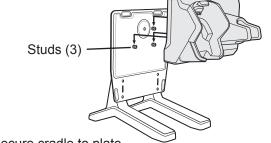
5. Secure cradle to plate using M3 safety screw.
