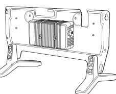
5. Align mounting slot on bottom of cradle with studs on plate.
