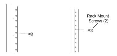
3. Align plate with the top two rack screws.
