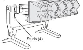
6. Secure cradle to plate using two M5 safety screws.
