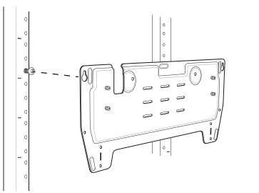
4. Install bottom two rack mount screws.
