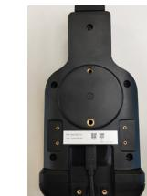
3. Insert the USB cover and fasten the screws.
