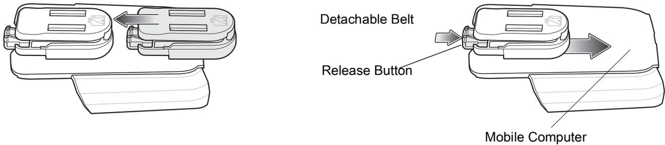
**Figure 67** Attaching the Rigid Holster
