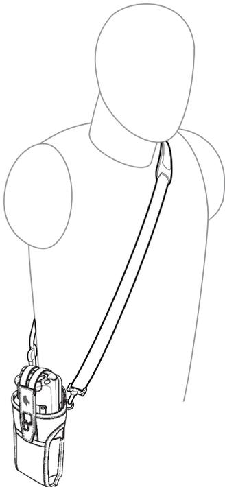
3. Lift the strap and insert the MC3300x-R/S into the holster.
