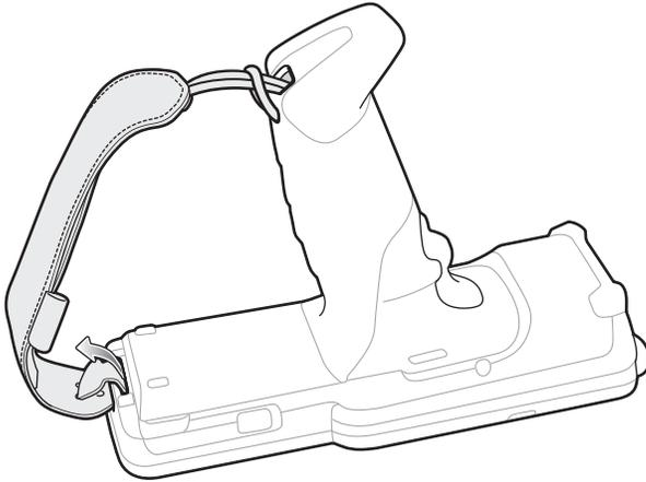
6. Slide the tab through the slit in the hand strap so that the tip of the tab is facing away from the MC3300x-G.
