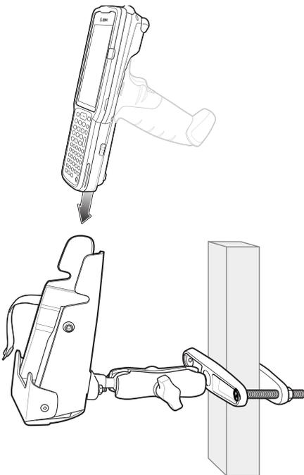
2. Secure the device with the rubber strap and snap into place.
