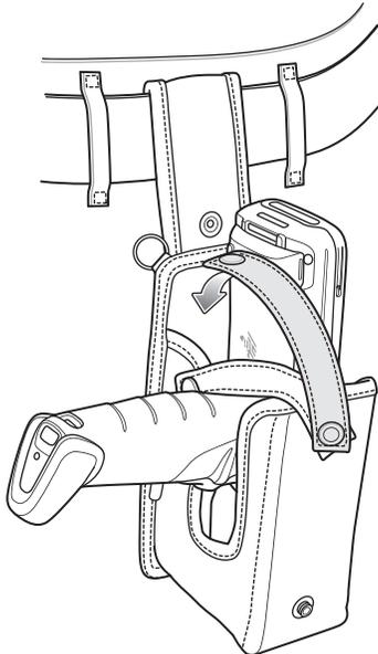
4. To remove the MC3300x-G, unsnap the restraining strap to release. Lift the MC3300x-G out of the fabric holster.
