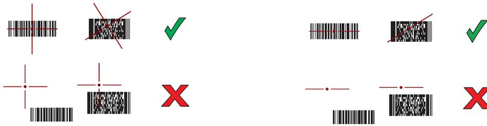
**Figure 21** Pick List Mode with Multiple Barcodes in Aiming Pattern: Standard and Extended Range
