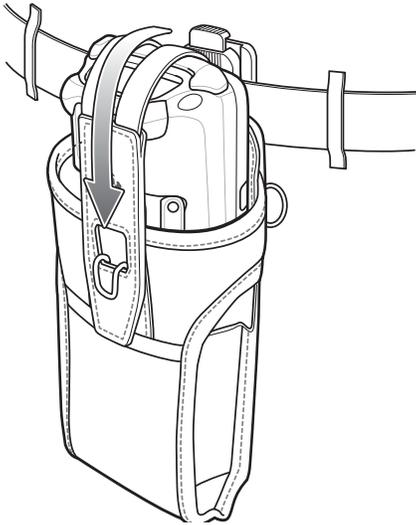
5. To remove the MC3300x-R/S, lift the restraining strap to release. Lift the MC3300x-R/S out of the fabric holster.
