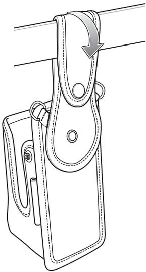
2. To insert the MC3300x-G, slide the mobile computer into the fabric holster with the screen facing the user.
