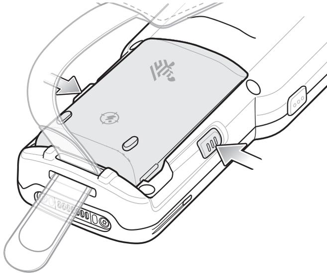
2. Remove the battery from the battery compartment.
