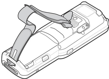
4. Pull the strap to the desired length and secure using the velcro.
