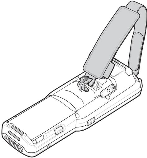
3. Thread the end of the hand strap with the velcro through the slot at the bottom of the MC3300x-R/S.
