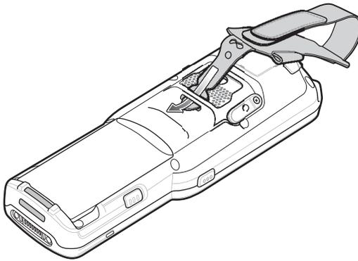
2. Slide the tab through the slit in the hand strap so that the tip of the tab is facing away from the MC3300x-R/S.
