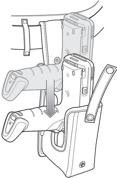
3. Secure the MC3300x-G with the restraining strap and place over the MC3300x-G to secure in place.
