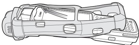
3. Grasp the bottom of the rubber boot and place over the bottom of the MC3300x-R.
