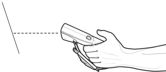
3. Press and hold the Scan button or Trigger.
