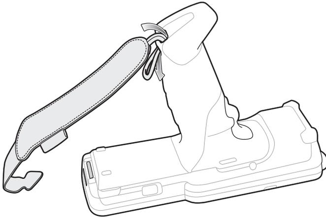
2. Insert the top end of the hand strap through the loop.
