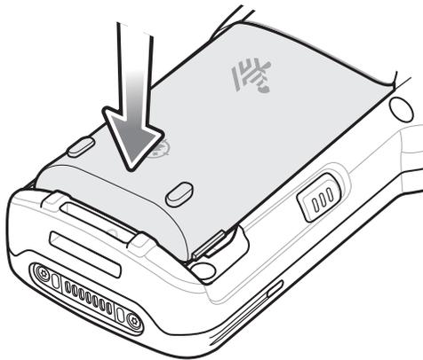
6. The device automatically resumes after a battery removal and installation (in a hot swap change). The only time the Power key needs to be pressed is if the device has been powered off or left for a prolonged duration without a battery pack.
