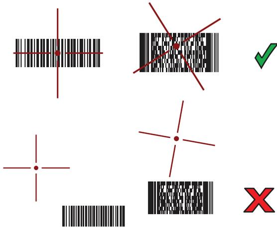
**Figure 26** RS6000 Pick List Mode with Multiple Barcodes in Aiming Pattern
