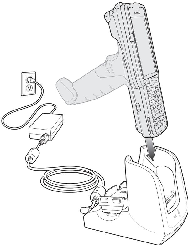
The MC3300x 7000 mAh PowerPrecision+ extended battery charges from 0% to 90% in less than 5.2 hours at room temperature.
