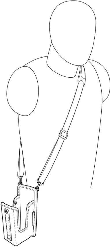
3. Lift the strap and insert the MC3300x-G into the holster.
