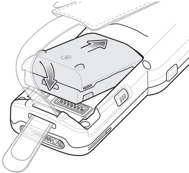
3. Slide the front of the battery into the battery compartment.
