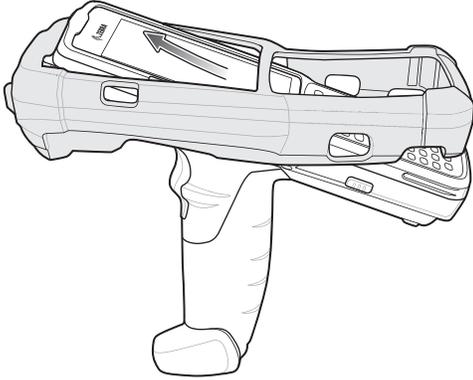
2. Grasp the bottom of the rubber boot and place over the bottom of the MC3300x-G.
