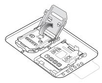
4. Place the nano SIM card into the card holder with contacts facing down.
