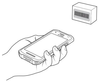
Press and hold the scan button. The red laser aiming pattern turns on to assist in aiming.
