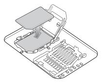
5. Close the SIM card holder door and slide into the lock position.
