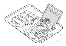
4. Insert the microSD card into the card holder door ensuring that the card slides into the holding tabs on each side of the door.
