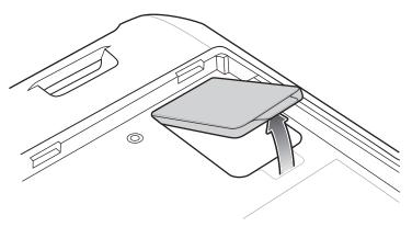
2. Slide the microSD card holder to the unlock position.
