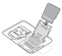
5. Close the microSD card holder and slide into the lock position.
