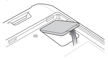
2. Slide the SIM card holder to the unlock position.
