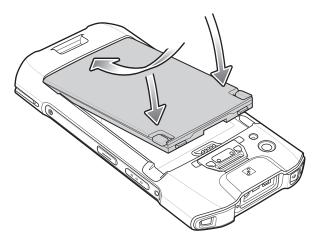
2. Press the battery down into the battery compartment until the battery release latches snap into place.
