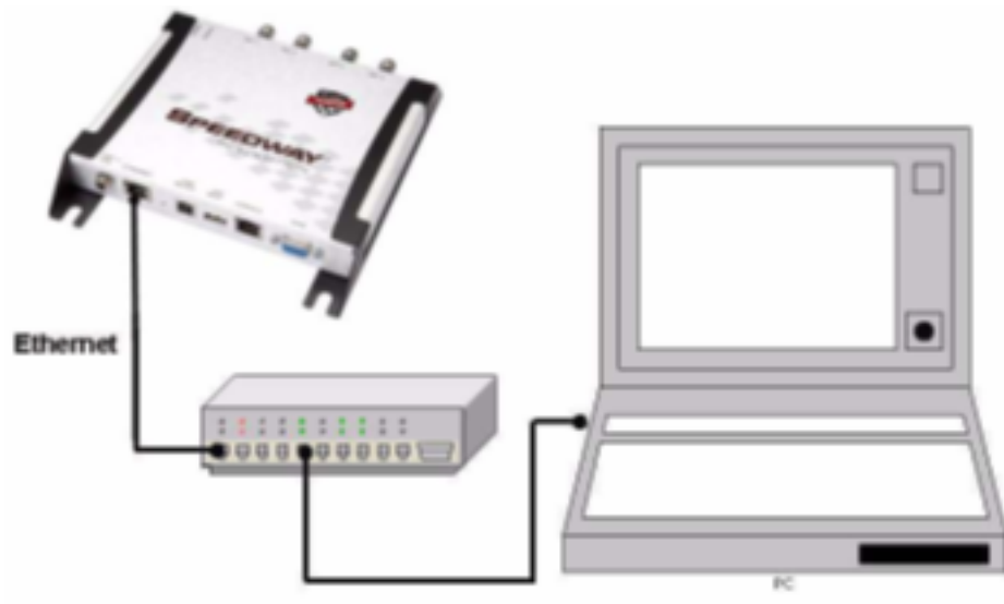
Figure 5.4 Connecting the Speedway Revolution Reader to the Ethernet Network
