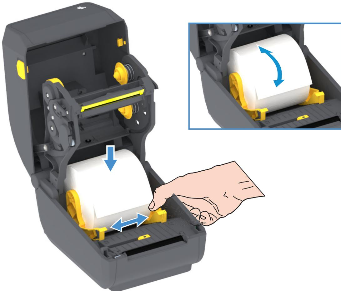
3. Pull the media so that it extends out of the front of the printer.
