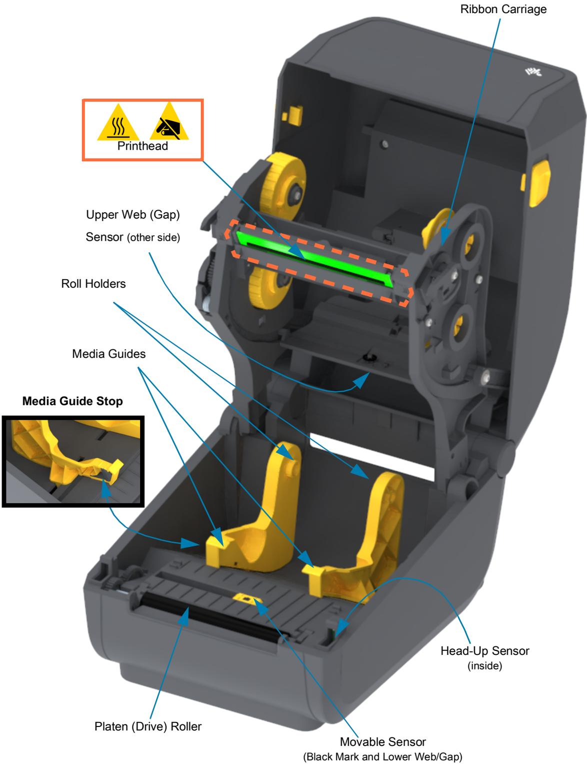
Dual Capacity Ribbon Chassis - Ribbon Roll Holders
