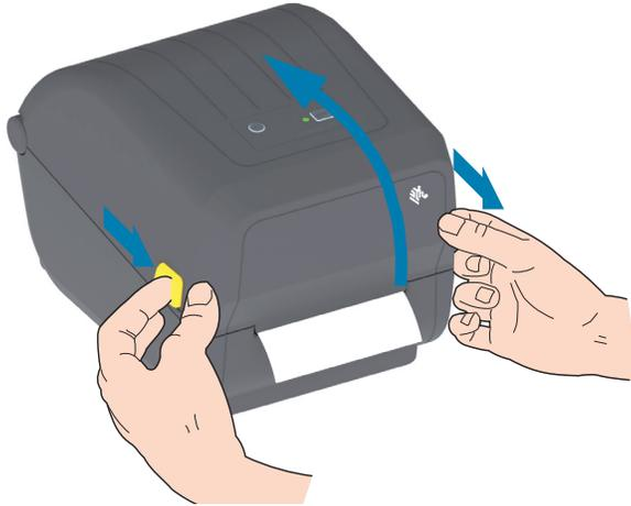
2. Open the media roll holders. Orient the media roll so that its printing surface will face up as it passes over the platen (drive) roller. Pull the media guides open with your free hand and place the media roll on the roll holders and release the guides. Verify the roll turns freely. The roll must not sit in the bottom of the media compartment.
