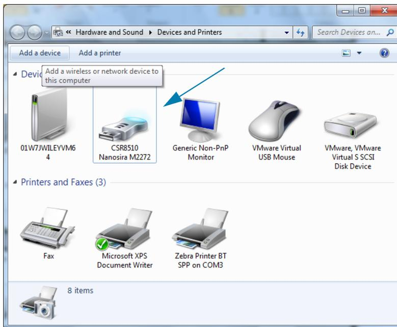
3. Hover over the Bluetooth icon with the mouse pointer and the icon will highlight. Right-Click on the high-lighted Bluetooth icon. Select 'Bluetooth Settings' from the pop-up menu. Verify that both of the Connections check boxes are checked. Verify that the 'Turn off the Bluetooth adapter' is not checked. Click the 'Apply' button. Click the 'OK' button to close the window.
