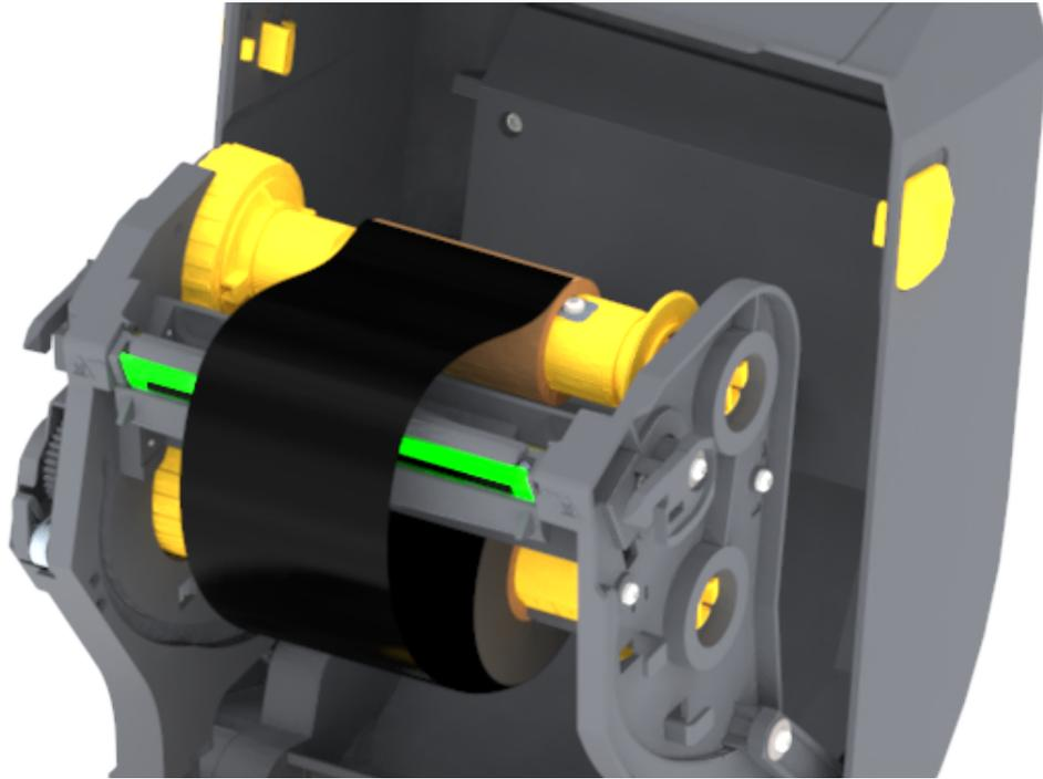
6. Turn the ribbon take-up hub with the top moving toward rear to remove slack from the ribbon. Rotating the hub helps to finish aligning the take up ribbon position with the supply ribbon roll. The ribbon should be wound, at minimum, one and a half times around the take-up ribbon core.
