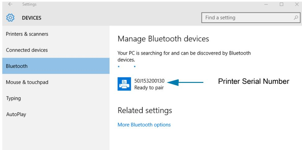
4. Click on the printer and then click on the 'pairing' button for the printer.
