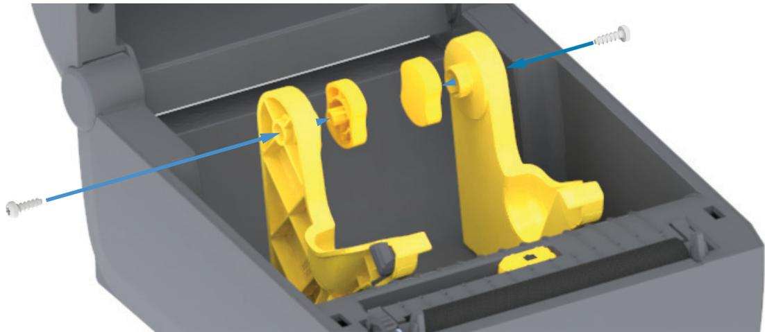
2. Place the adapter on the inside of the roll holder. The large side of the adapter is on top. The smooth side (no ribs) faces the middle of the printer.
