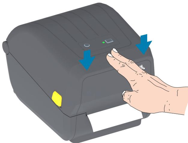
You may need to calibrate your printer for the media. The printer's sensors need to adjust to sense the label, the liner, and the distance between labels to operate properly. When reloading the same media (size, vendor, and batch), you can just press the FEED (Advance) button once to prepare the media for printing.
