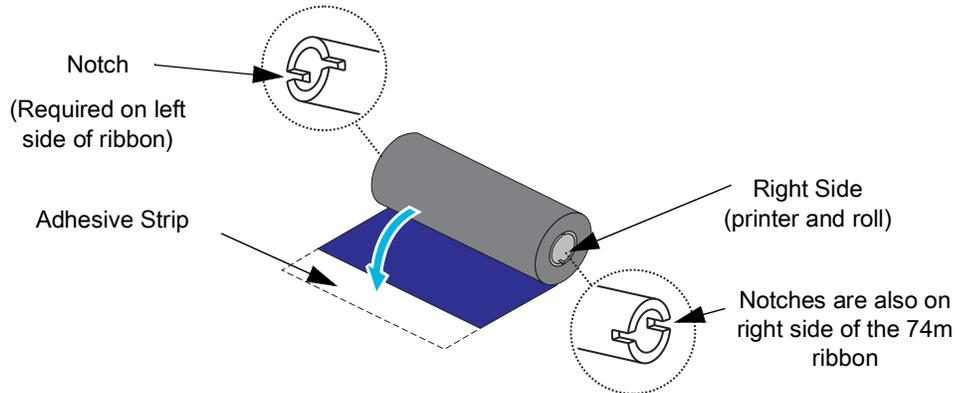
Verify that the ribbon and empty ribbon core have notches on the left side of the ribbon cores as shown above. If they do not, see [Loading Non-Zebra 300 Meter Transfer Ribbon](#).
