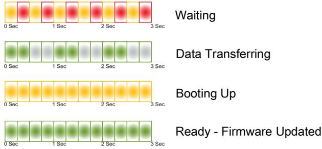
The STATUS Indicator alternates Amber and Red. If you release the FEED button here, the printer begins waiting for data to begin download (of the printer firmware file).
