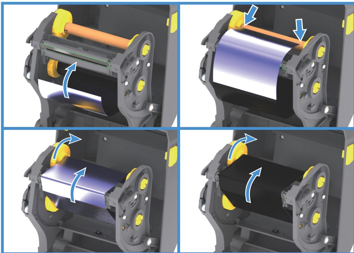
4. Turn the ribbon take-up hub with the top moving toward rear to remove slack from the ribbon. Rotating the hub helps to finish aligning the take up ribbon position to the supply ribbon roll. The ribbon leader should be completely covered by the ribbon.
