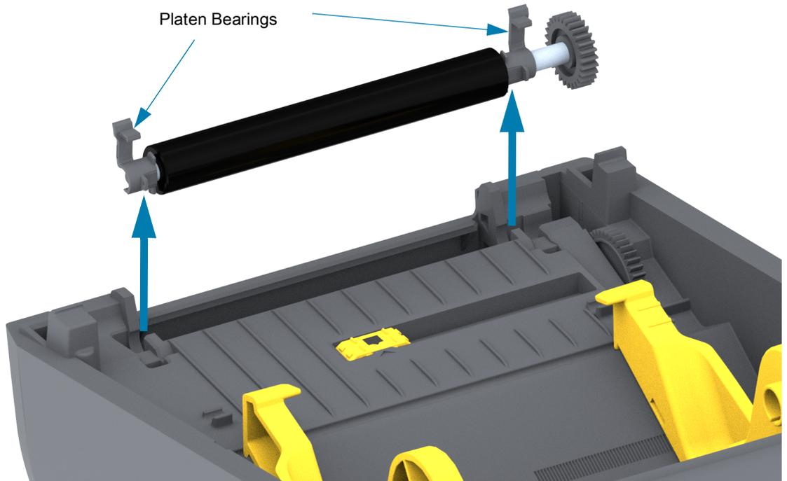
4. Slide the gear and the two (2) bearings off the shaft of the platen roller.
