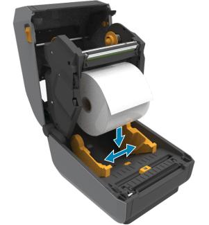
Spread the roll holders open and place the roll into the printer.
