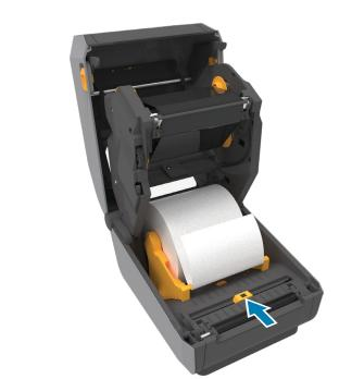
Align the sensor to the center of the roll for regular labels.
