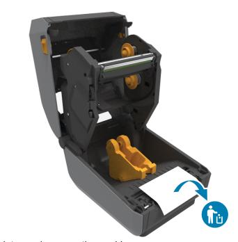
Open the printer and remove the packing.
