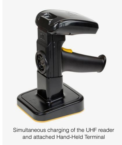
Simultaneous charging of the UHF reader and attached Hand-Held Terminal
