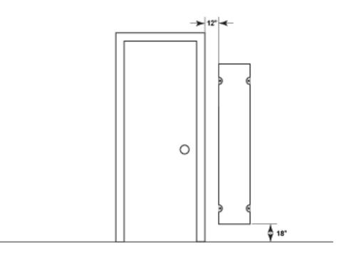
b. Do not mount the panel on the hinge side of the doorway. This could cause damage to the antenna from door impacts.
