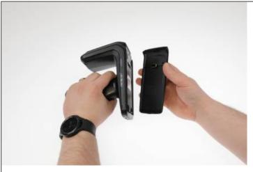
2. **Remove Top Cover:**Once loose, the top cover can be removed completely and set aside for any future
