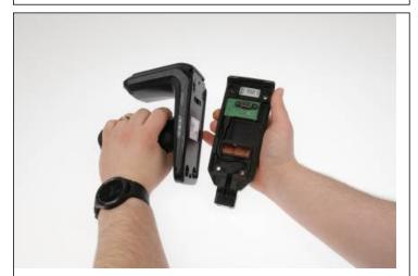
3. Align the Adapter Plate: This adapter plate is designed to fit into the RFD40 exactly to seal the product and securely fasten to it. Align the 4 screw holes with the top of the RFD40.
