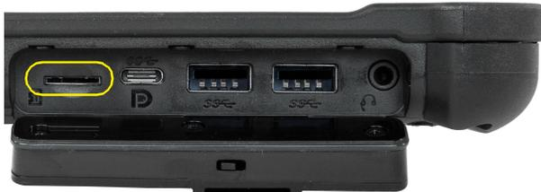
2. Use the stylus tip on the tablet pen and insert it into the reset hole to press the recessed button until the tablet shuts down. (You can also use a paper clip and unbend it to form a pin.)
