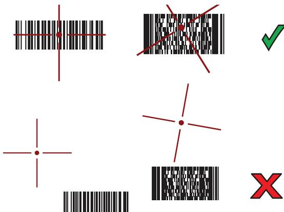
**Figure 27** RS507/RS507X Pick List Mode with Multiple Barcodes in Aiming Pattern
