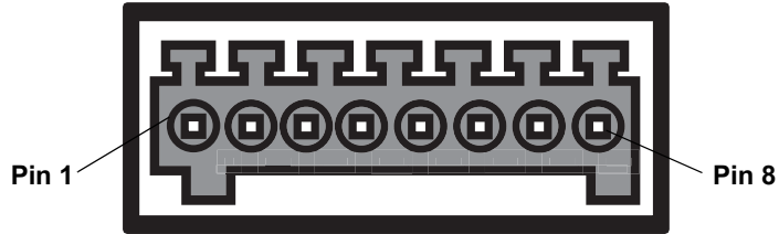
Figure 96 FX7500 RFID Reader GPIO Connection
